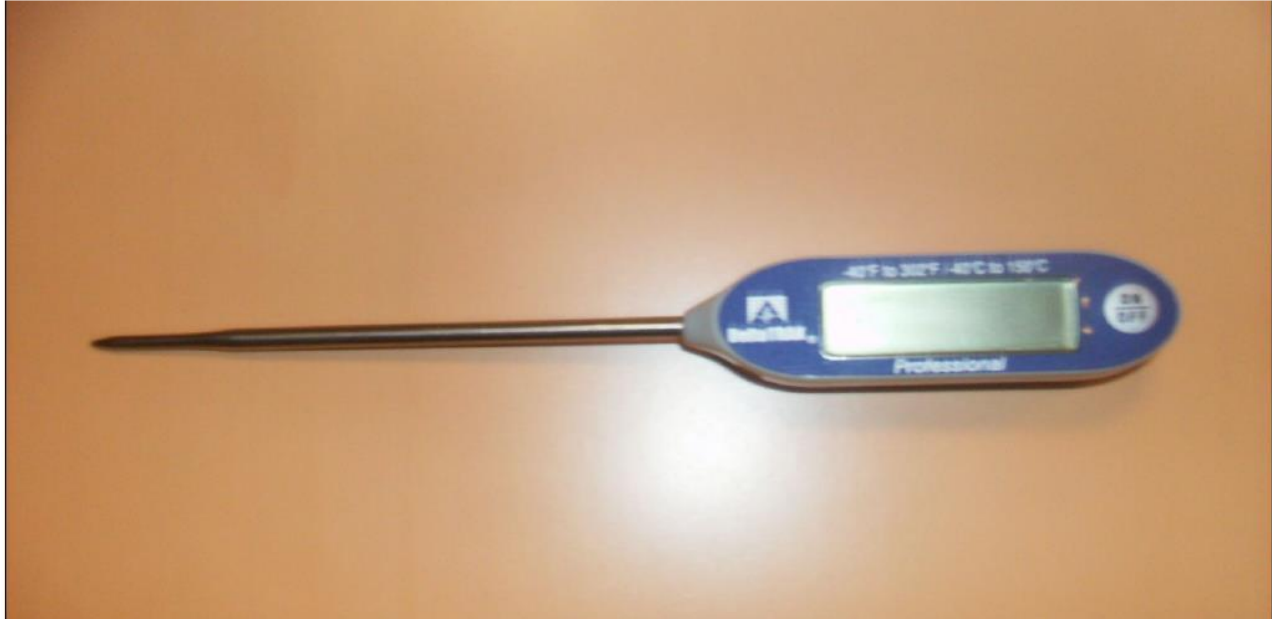
Picture 2: Digital thin-tipped PROBE thermometer for taking food temperatures.
